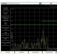
DTF is a way to locate faults identified by Return Loss or VSWR measurements.
