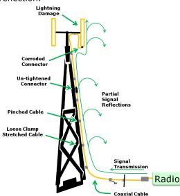
Changes in impedance, in turn, are caused by mismatches, or physical changes in the cable, such as:
